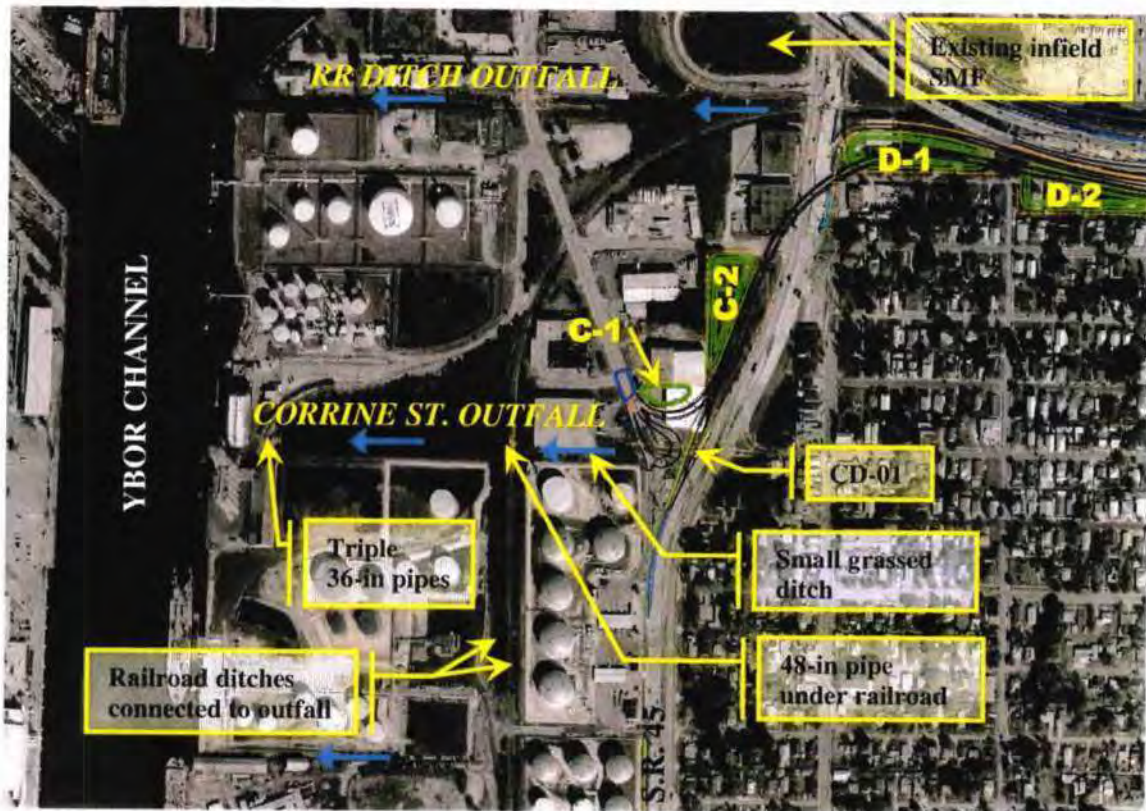
Figure 4.4.1 – Outfalls to Ybor Channel
